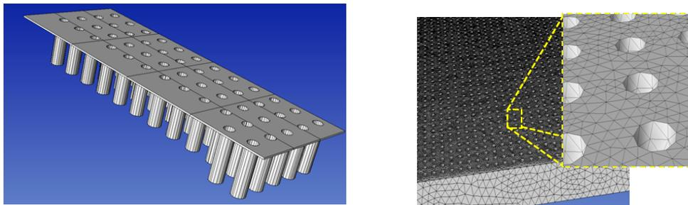
*Figure 1. Geometric model of liner film (left) and a 1.1 billion element mesh generated in parallel with Simmetrix SimModSuite on AMOS BG/Q (right).*
