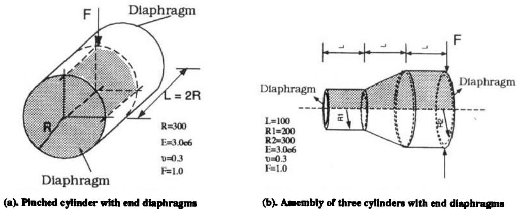
Figure 1. Geometry, boundary conditions, material properties
