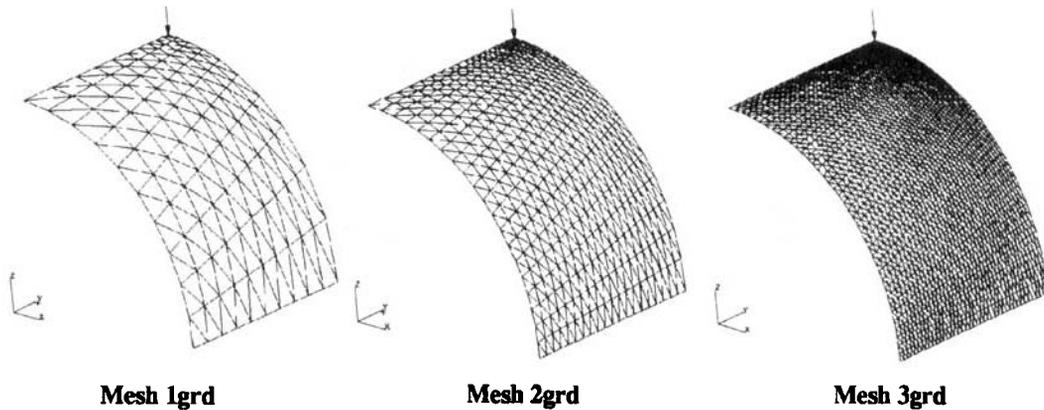
Figure 2. Graded mesh information (flat shell triangular)
