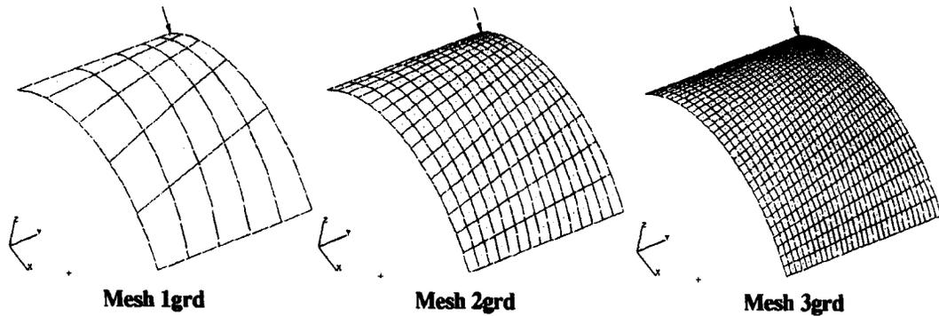
Figure 3. Graded mesh information (quadrilateral shell element)
