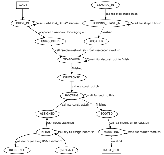
Figure 4: RSA state change diagram for Running jobs.
