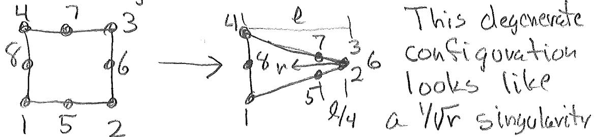
Linear fracture mechanics says there is a  $1/\sqrt{r}$  strain singularity at the crack tip. Use the above degenerate 8-noded hexes and it mimics the  $1/\sqrt{r}$  singularity - Used all the time for fracture analysis
